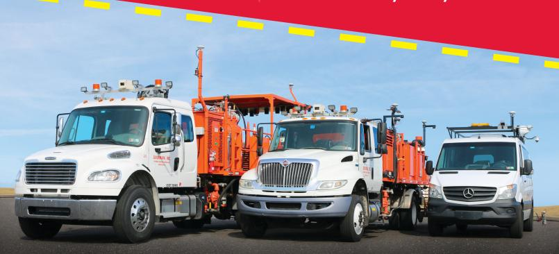
THE LIFEMARK™-75 AUTOMATED LAYOUT SYSTEM was designed specifically for the roadway stripers market. Using real-time kinematics (RTK) enhanced GPS-based location and laser technologies, this system provides stripers with the ability to accurately record the location of roadway markings before the roadway is repaved. Once the roadway is repaved, the original markings can then be duplicated in the same GPS location with workers safely off the road and out of harm's way.
