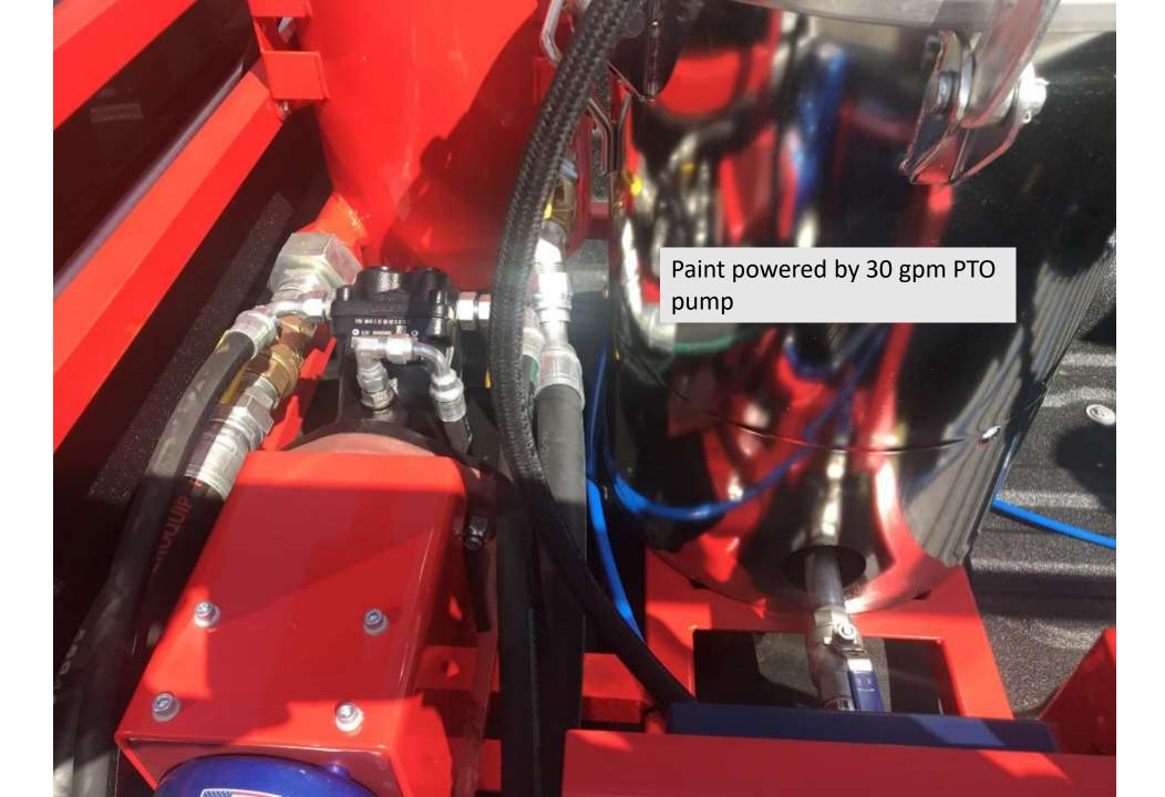
30 gallon per minute PTO pump mounted to transmission
